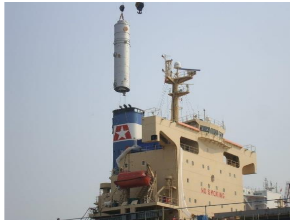
The new scrubber tower during descent in the existing funnel at the yard
